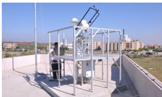
Meteorological High Precision (MPH) Solar/Wind measuring Station
